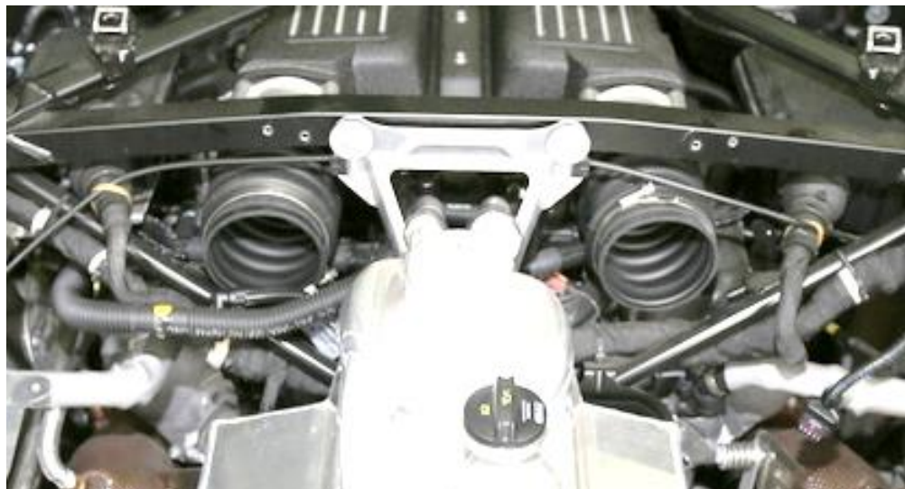
16. Remove both of the flexible rubber hoses from the throttle bodies.
