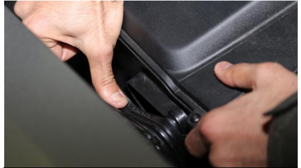
10. Push the plastic inlet duct connectors off the airboxes. They are located on the side of the airboxes nearest the wing. If you have an EVO or STO you will have to remove the round duct connectors from the feeds.
