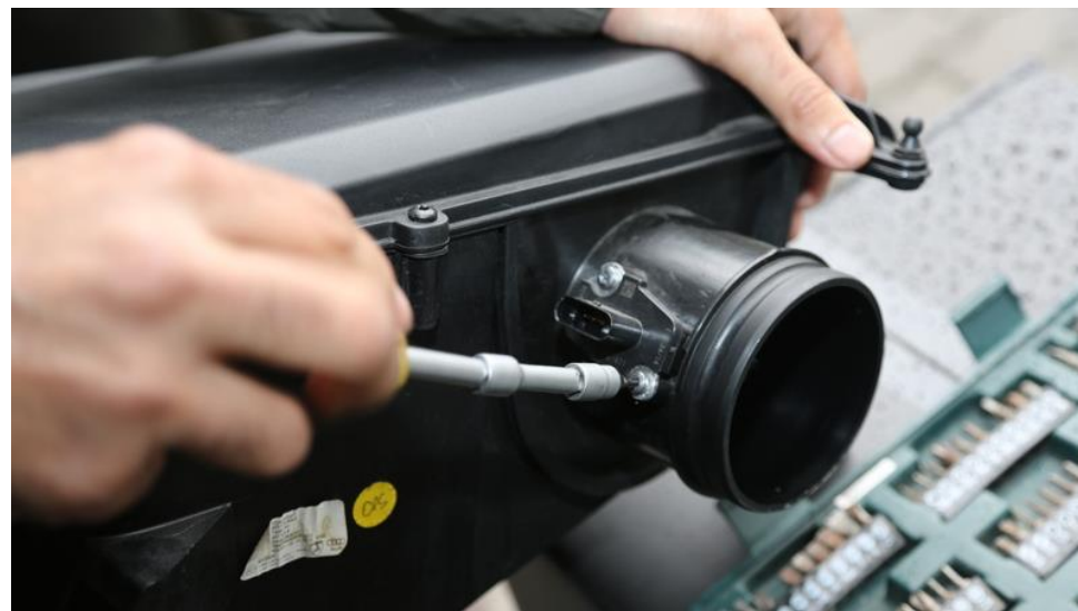
14. Remove the MAF sensors from the original airboxes. They are held in place with 2 screws.
