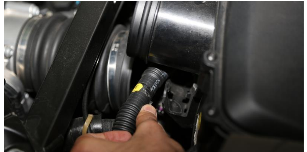
12. Now the airboxes can be pulled out. On the left airbox (as you look at the engine) there is a hose which needs to be removed from the airbox as shown. Remove both airboxes completely. On the Audi R8 you will need to disconnect the vacuum line to the secondary flaps on the airbox. We will plug this later.
