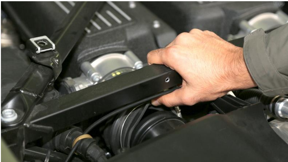
11. Loosen the hose clamp around the inlet tubes and push them off both airboxes.
