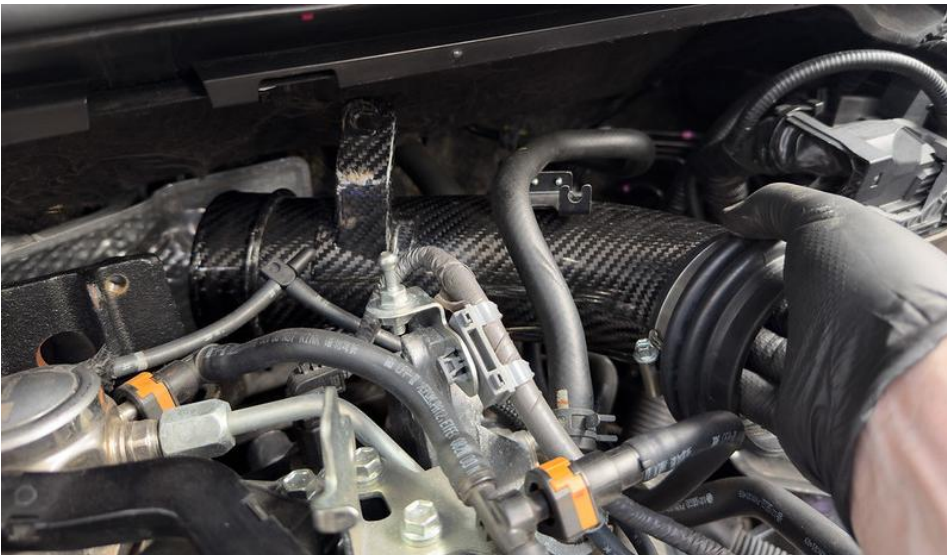
11. Remove the rear intake tube. (Carbon version shown here from the Corolla system).
