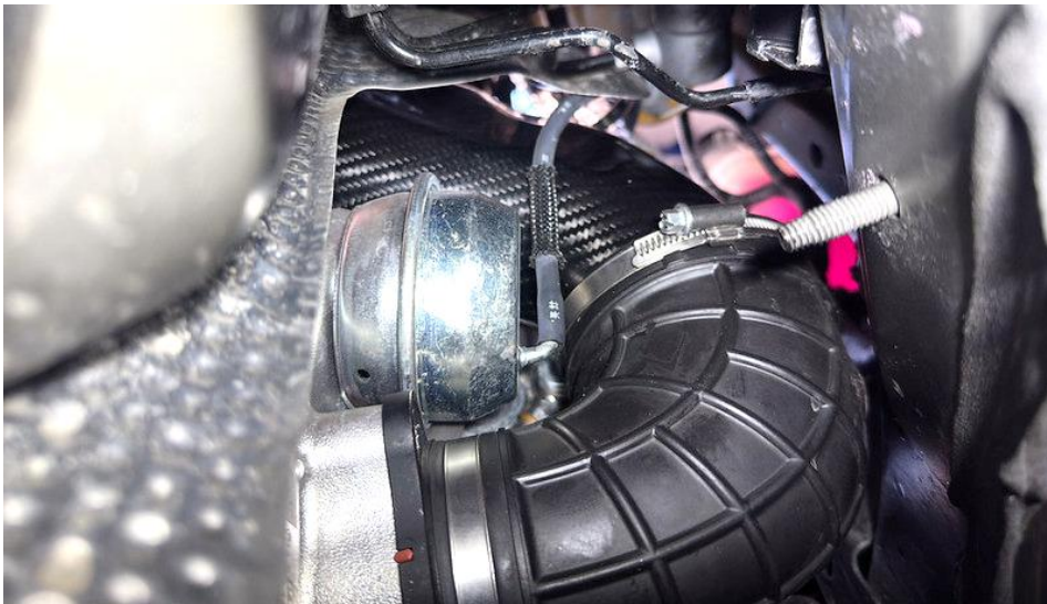
26. Push the tube into the rubber elbow – make sure it is fully engaged into the elbow. The hose clamp should be very loose to allow this. Do not tighten yet.
