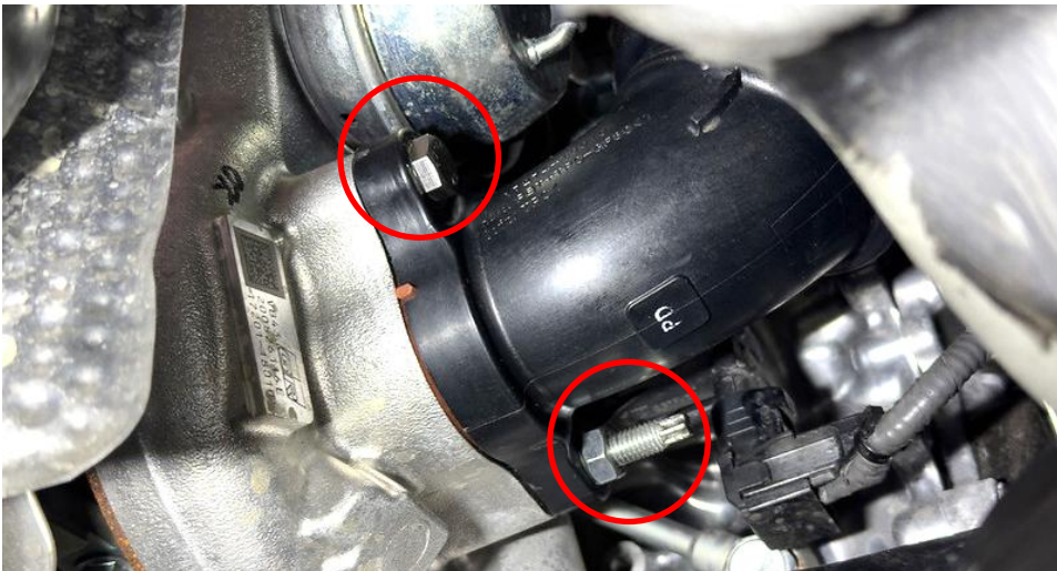
15. Now you can access the OEM turbo elbow. Remove the 13mm bolt on the left and the nut on the right.
