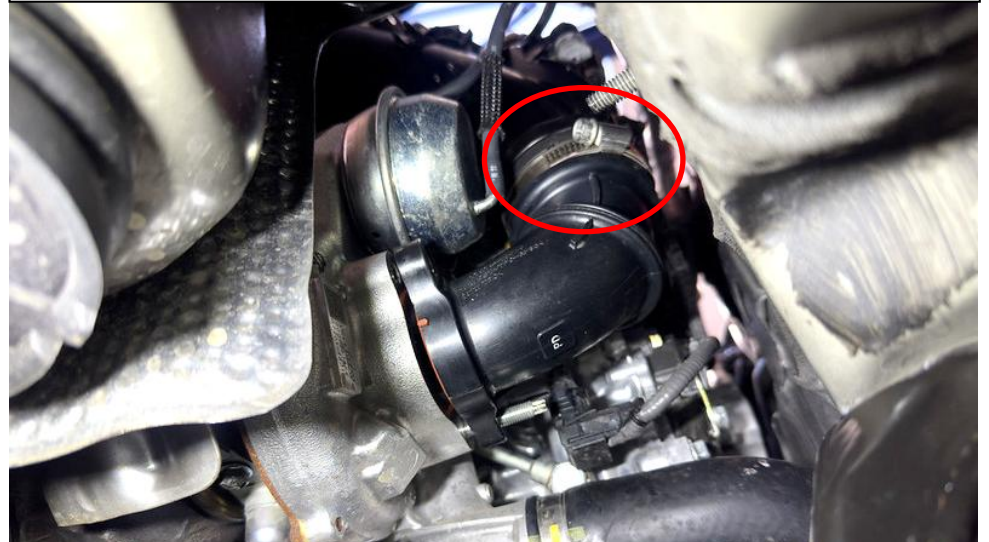
16. Loosen the hose clamp between the elbow and the upper tube. Then you can remove the elbow from the turbo.
