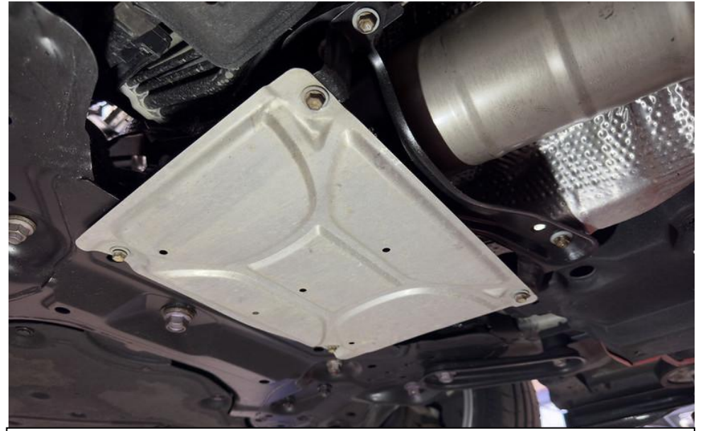
14. Remove the metal undertray. There are 4 x 10mm bolts holding it in place.
