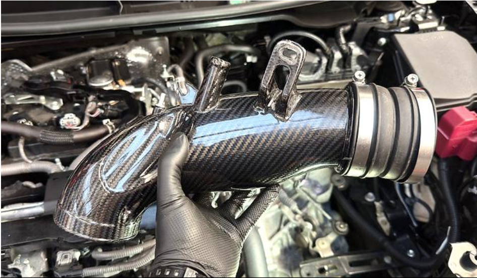
24. Install the OEM rubber coupler to the Eventuri turbo tube.
