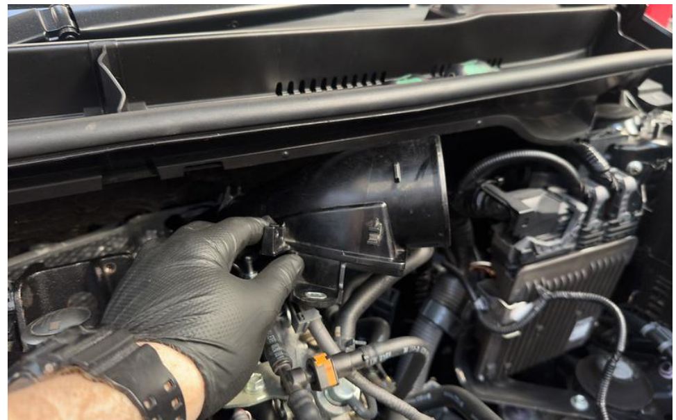
19b. Remove the vacuum lines held on the tube and then you can remove the tube. The tube will have a rubber coupler on the end of it – remove this for use later.
