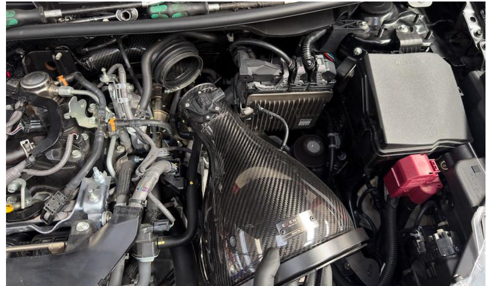
8. You can now remove the filter housing.
