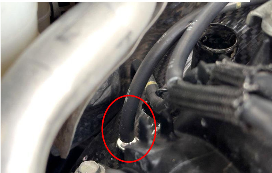
13. Remove the vacuum tube from the top of the turbo tube.
