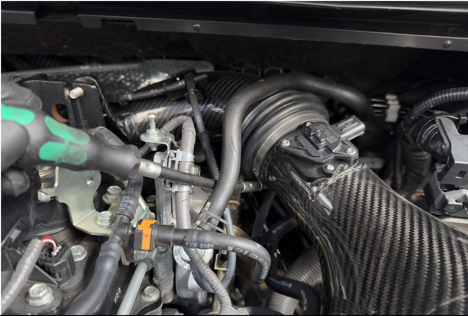
5. Loosen the hose clamp at the back of the intake housing.
