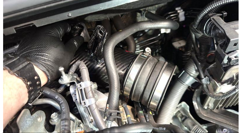
25. Slide the tube into position from the intake side of the engine.
