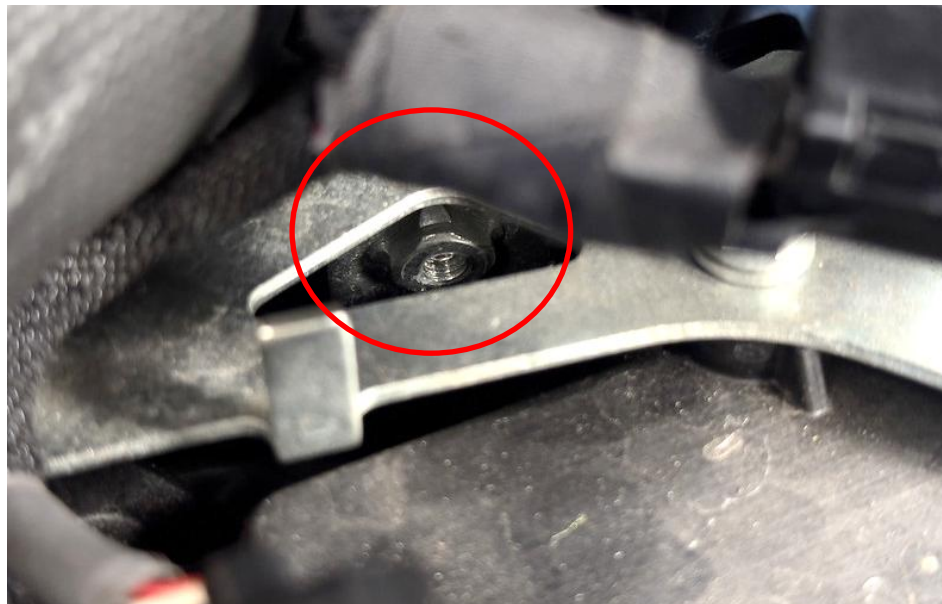
19. The bolt holding the turbo tube is located here – remove the bolt using a 10mm socket.
