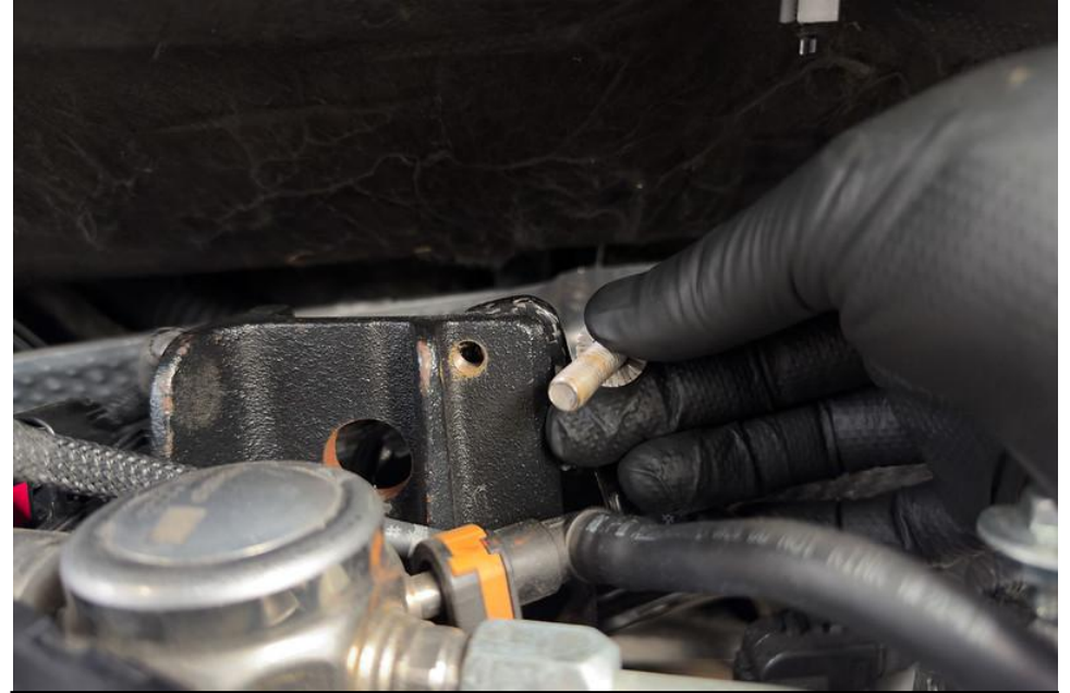
6. Remove the M8 bolt holding the rear intake tube in place. Make sure you also remove the locking washers with the bolt. They will need to be re-used.
