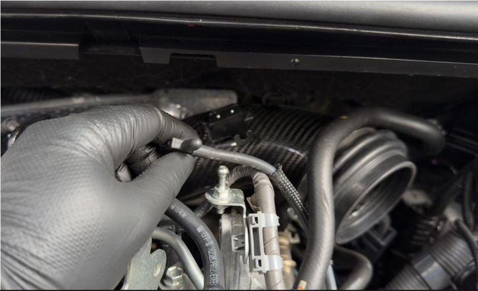
9. Remove the vacuum line junction from the rear intake tube.
