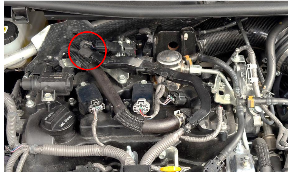
18. The upper turbo tube is secured in place with a 12mm bolt behind the engine in the area shown. See next photo for a close up.
