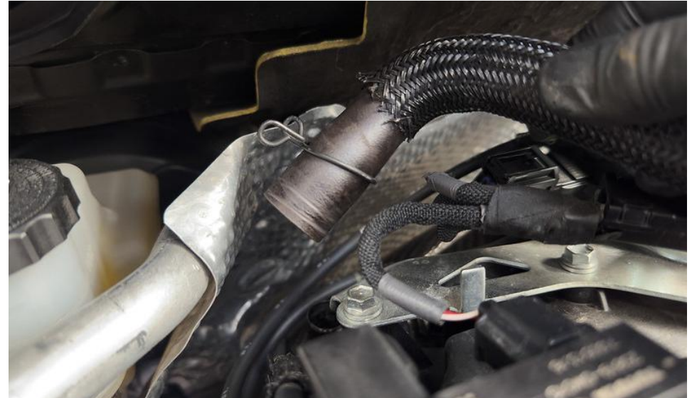
12. Remove the breather hose from the turbo inlet tube – compress and pull the clamp around it upwards and then you can pull it off.
